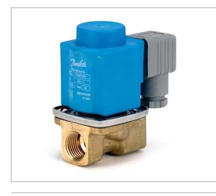
EV220B 6 - EV220B 22 is a direct servo-operated 2/2-way solenoid valve program with connections from 1/4" to 1". This program is especially for OEM applications demanding a robust solution and moderate flow rates.
