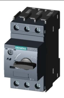
CIRCUIT-BREAKER SZ S00, FOR MOTOR PROTECTION, CLASS 10, A-RELEASE 7...10A, N-RELEASE 130A, SCREW CONNECTION, STANDARD SW. CAPACITY
