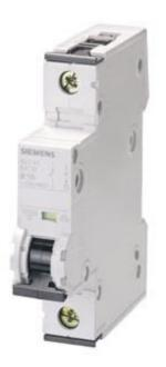
CIRCUIT BREAKER 230/400V 6KA, 1-POLE, C, 2A, D=70MM
