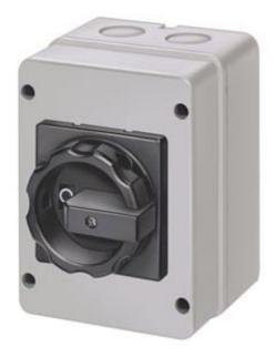
MAIN CONTROL SWITCH 3-POLE IU=25, P/AC-23A AT 400V=9,5KW 1 N-TERMINAL + 1 PE-TERMINAL ENCAPSUL.IN M.P.ENCLOSURE, IP65 ROTARY ACTUATOR BLACK METRIC THREAD
