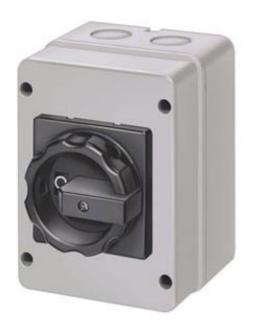
MAIN CONTROL SWITCH 3-POLE IU=63, P/AC-23A AT 400V=22KW 1 N-TERMINAL + 1 PE-TERMINAL ENCAPSUL.IN M.P.ENCLOSURE, IP65 ROTARY ACTUATOR BLACK METRIC THREAD
