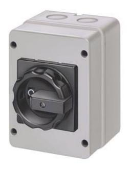
3-P. MAIN CTR. SWITCH IU=16, P/AC-23A AT 400V=7.5KW 1 N-TERMINAL + 1 PE-TERMINAL MOULDED-PLASTIC ENCLOSED, IP65 ROTARY ACTUATOR BLACK
