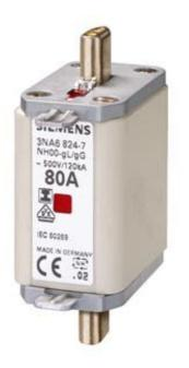
LV HRC FUSE LINK GL/GG WITH INSULATED GRIP LUGS WITH COMBINATION INDICATOR SIZE 00, 125A, AC 500V/DC 250V
