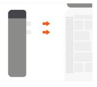
Connect external monitor to HDMI port on the Hub. Use HDMI-HDMI cable version 1.4 or higher. Available quality 1080p @ 60Hz, up to 4K @ 30Hz
