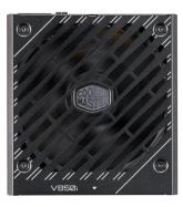
The 135mm silent fan creates less friction, making it great for low RPM operations while delivering quiet cooling performance.
