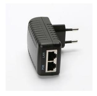
With the Auerswald PoE Injector, an IEEE 802.3af-compatible network device, such as a Wireless Access Point, IP telephone, or network camera, can be supplied with power directly over the network cable. This means it can also be connected using devices that are supplied by the network cable to a LAN switch port without a feed point.
