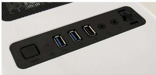
- I/O-Panel with: 2x USB 3.0 port, 1x USB 2.0 port, HD Audio, fan speed control
