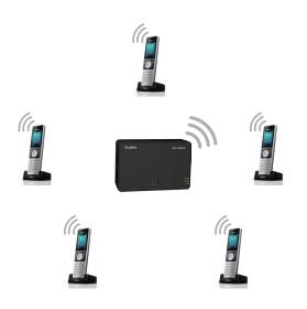
The W56P systems can be expanded up to a total of 5 cordless handsets by adding the W56H or W52H cordless handsets
