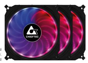
by switching with corresponding + 5V LED headers. Each fan is equipped with 16 addressable LEDs and allows an almost infinite RGB effect variety which cannot be realised by a simple and conventional +12V RGB lighting.
