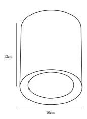
Voltage (V): 230 Volt IP degree: IP20 Class (Class 1, Class 2, Class 3): Class 2 (Double isolated) Bulb base: LED Module Parallel connection: True
