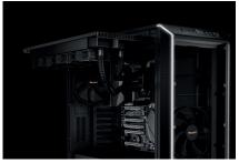
Cooling-optimized: The two pre-installed and virtually inaudible SilentWings® 3 PWM fans provide excellent air circulation. A removable bracket is provided to mount the optional fans or radiators on before installing the completed unit into the case. Perfect for water cooling with radiators up to 360mm.
