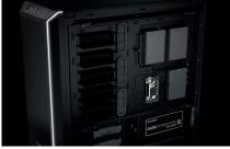
**Perfect compatibility:** Flexible installation, thanks to repositionable single HDD slots. The multifunctional PSU shroud offers space to hide drives and cables. Supports up to three HDDs or nine SSDs.
