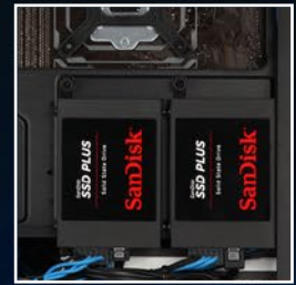
Mounting Bracket for up to Two 2.5" HDD/SSDs
