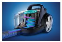
The aerodynamic design of PowerCyclone 7 minimizes air resistance and ensures exceptional cleaning performance through 3 highly efficient steps: 1) Air enters fast into the PowerCyclone thanks to the straight and smooth air inlet. 2) The curved airpass quickly accelerates the air upwards in the cyclonic chamber. 3) At the top of the cyclone, the exit blades effectively cut out the dust from the air.
