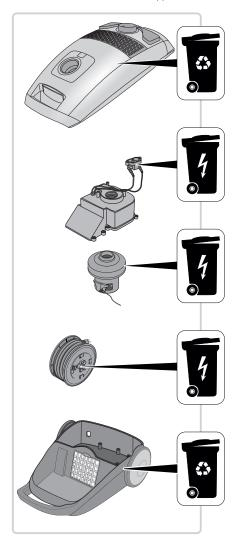
Loosen all screw connections and other connections until the appliance components can be disposed of separately as follows: 0
