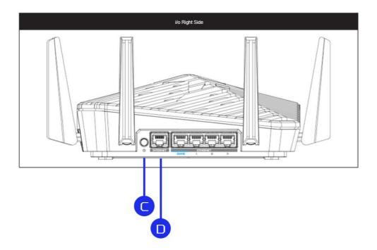
C: Push the Power Button located on the rear right side. Once turned on, the Predator Connect W6 Wi-Fi 6E Router's LED will light up. Please refer to the LED indicator table on page 4 for more information.
