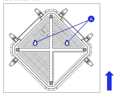
A: 2 Wall Mount Holes in blue outlines at 10cm or 4inches wide. Follow the reference image above for correct orientation and proper device mounting. Note:
