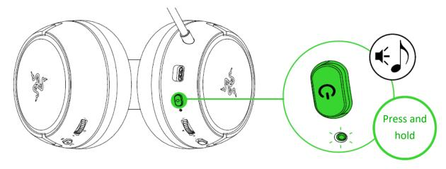
3. Wait until the status indicator briefly becomes static green indicating that the headset is now connected to the Type-C wireless dongle.
