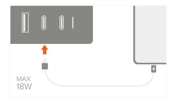
Fast charge USB-C PD devices using an Apple MFi-Certified USB-C to Lightning cable.
