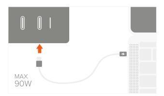
4 Connect a Type-C smartphone or tablet to the second USB-C PD port.
