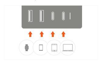
3 Connect a Type-C laptop or tablet to the first USB-C PD port.
