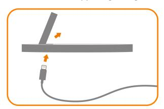
**5.** Press the cable into the trough on the bottom of the base.
