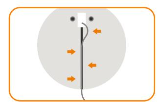
2. Tighten the two hex screws on the bottom of the base using the included allen wrench.
