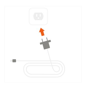
2 Connect the Wireless Charger V2 to Type-C power adapter.
