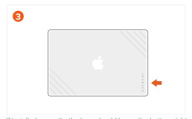
If installed correctly, the logo should be on the bottom right.
