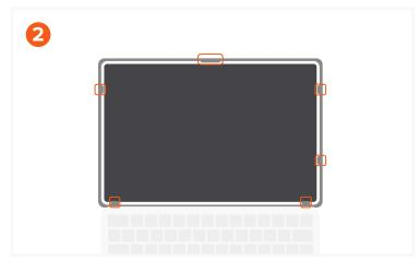
When installing the top case, ensure all **6 clips** snap into place.
