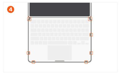
When installing the bottom case, ensure all **7 clips** snap into place.
