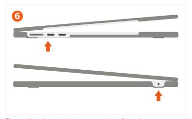
Ensure that the cutouts are properly aligned.
