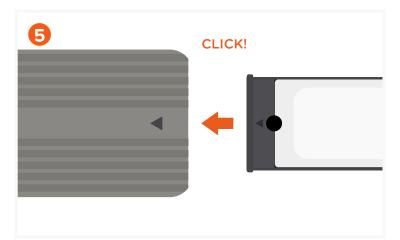
Once the SSD is secured, align arrows, and push into the enclosure. You should hear a clicking sound once the internal enclosure is locked into place.
