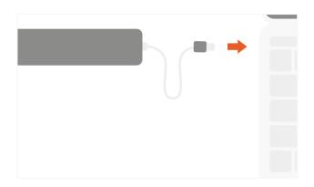
2 Connect an USB-C charging cable to the adapter's USB-C PD charging port.
