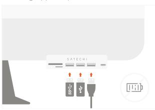
2 Attach the hub to the bottom right side of your iMac (same side as ports) and turn the knob clockwise to tighten.
