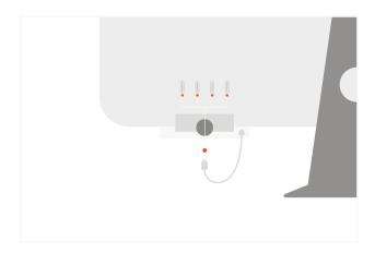
**5** Connect USB-A thumb drives or peripherals to its three USB-A 3.0 data ports.
