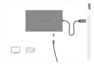
5 Use the two USB-A 3.0 ports for data transfer and file back up – up to 5 Gbps. USB-A ports do not support charging or CD readers, including Apple SuperDrive.
