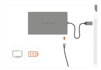
4 Use the USB-C data port to connect an USB-C device or peripheral – up to 5 Gbps.
