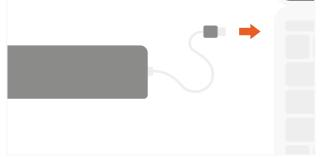
Use HDMI cable to connect external monitor to HDMI port. Display will be mirrored on HDMI monitor.
