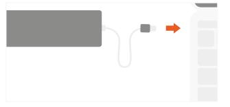
Connect external monitor to HDMI port of the Adapter with HDMI Cable.
