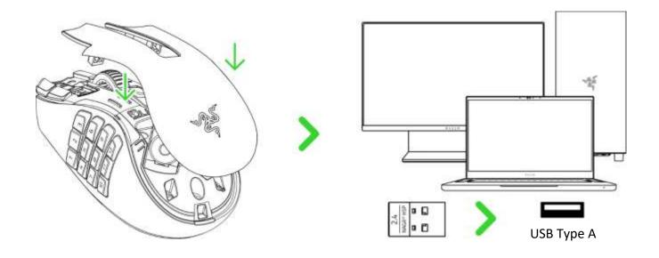
3. Push the slider switch to Razer™ HyperSpeed Wireless (2.4 GHz) mode. When connected, the status indicator will briefly turn static green.
