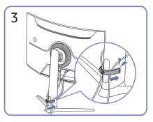
Put both cables in the cable holder on the stand (HOLDER-STAND CABLE) to organise the cables, as shown in the figure. Assembly is complete.
