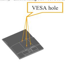
Step 5: Attach the LCD display to the wall, following the instructions in the wallmounting kit. For use only with UL/GS Listed Wall Mount Bracket with minimum weight/load: 10.95 kg
