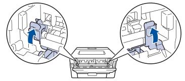
If you print on envelopes, pull down the green envelope levers to the envelope position again before closing the back cover.
