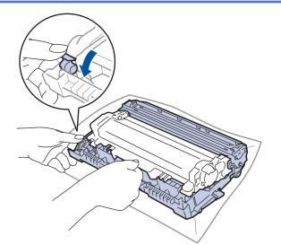
10. Turn the drum unit as shown in the illustration. Make sure that the drum unit gear (1) is on the left side.
