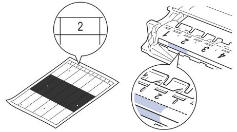
12. Turn the drum unit edge towards you while looking at the drum surface to find the mark.
