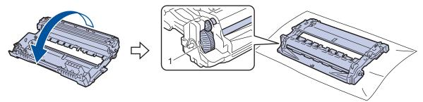
8. Use the numbered markers next to the drum roller to find the mark on the drum. For example, a dot in column 2 on the check sheet means that there is a mark in drum region "2".
