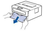
Pulling the jammed paper downwards using both hands allows you to remove the paper more easily.
