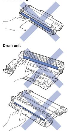
(For certain models) The toner cartridge features an IC chip. DO NOT touch this surface. Touching the IC chip may cause contamination or damage, and may interfere with the machine's ability to detect this component.
