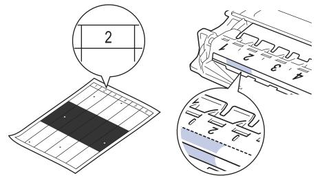
9. Turn the drum unit edge towards you while looking at the drum surface to find the mark.
