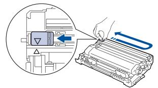
Be sure to return the tab to the Home position ( $\blacktriangle$ ). The arrow on the tab must be aligned with the arrow on the drum unit. If it is not, printed pages may have a vertical stripe.
