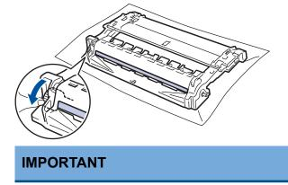
To avoid print quality problems, DO NOT touch the surface of the drum unit, only the wheel on the end.
