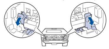
If the green envelope levers inside the back cover are pulled down to the envelope position, lift these levers to the original position before pulling the blue tabs down.
