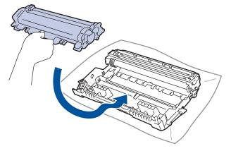
$^\prime$  Make sure you put the toner cartridge in correctly or it may separate from the drum unit.
