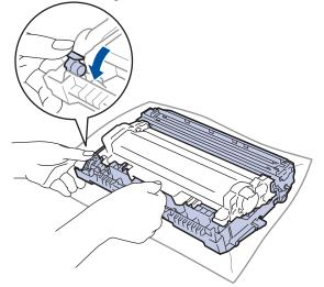
7. Turn the drum unit as shown in the illustration. Make sure that the drum unit gear (1) is on the left side.
