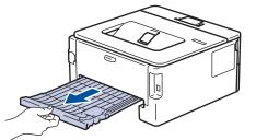
4. Pull the jammed paper out of the machine or out of the 2-sided tray.
