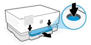
2. Remove the input tray by pulling it all the way out of the printer.
