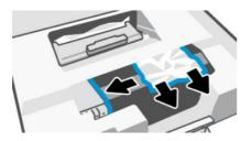
4. Lift the handle of the paper path cover and remove the cover.
