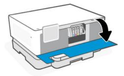
2. Open the cartridge access door, and then wait until the carriage stops moving.
