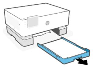
3. Check the input tray area underneath the printer. Remove any jammed paper.
