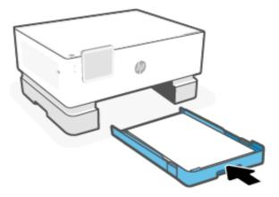
5. Insert the output tray back into the printer.
