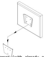
Engage a screen (with already attached front plate) to the back plate on wall.
