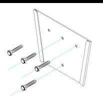
Mount back plate in desired position using screw/bolts
