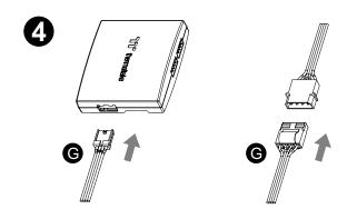
Connect the power cable to the 4pin Molex connecter and controller.
