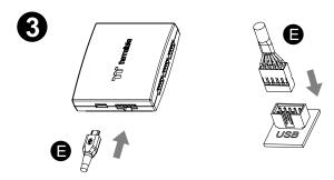
Connect the controller cable onto the motherboard (USB 2.0 9 pin) and controller.
