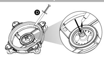
After replacing the fan blades several times, readd the oil into the bearing (about 0.1ml)
