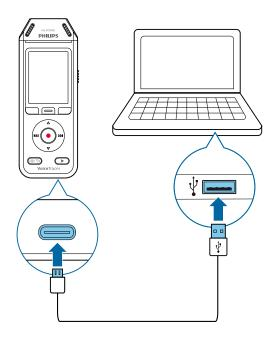
→ A charging battery icon appears on the screen and the Record/Status LED flashes orange for a few seconds.
