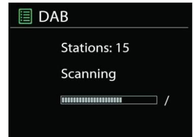
To start the scan, press the "MENU" button on the remote control or press and hold the "MENU / INFO" button to access the DAB menu. Select the option "Full scan" and confirm with "OK" or press the "SCAN" button on the remote control.
