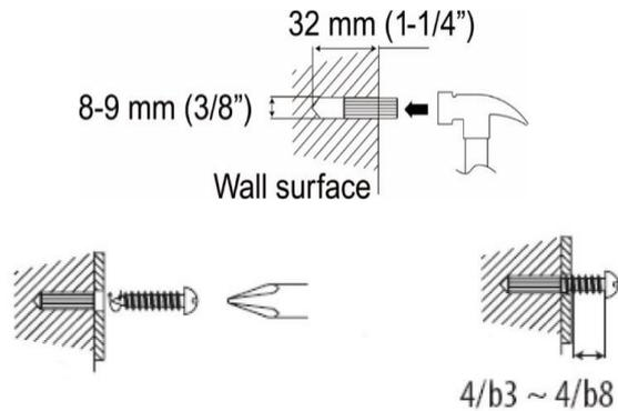
Remove the base of the device by pulling the two locks on the underside of the base away from the device. Push the stand foot back and pull it off. Now you can hang up your device as shown in the picture
