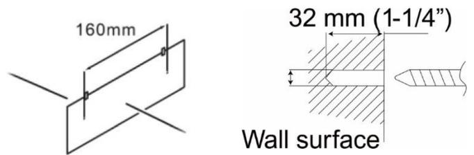
Attach the screws with proper dowels as you can see in the pictures
