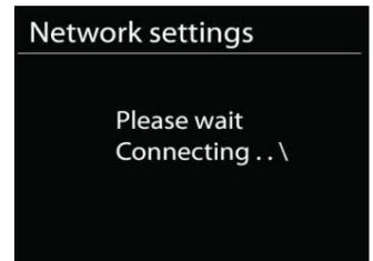
It will show connected if the setup is successful. If connecting fails, ICD1010 returns to a previous screen to try again.
