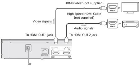
→ If selecting this connection method, set [HDMI Audio Output] in [System Settings] to [HDMI2] or [Auto] (page 25).
