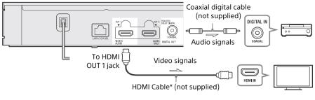
→ If selecting this connection method, set [HDMI Audio Output] in [System Settings] to [HDMI1] or [Auto] (page 25).
