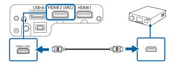
• To output audio from the projector's HDMI2 (ARC) port, set **HDMI2 ARC** to **On** and **Sound Output Device** to **ARC** in the projector's menu.
