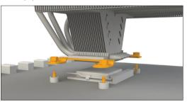
and affix by turning the AMD M3x15 screws (10) from the rear side of the motherboard.
