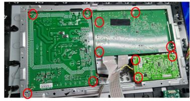
Remove the usb Remove the screw on the usb board board Remove the 3pcs screws on the keyboard Remove the keyboard Remove the Remove the screws on the middle frame middle frame Mainboard and powerboard and coverter board
