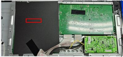
Remove the powerbard and mainboard and converter board
