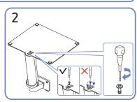
Tightly fasten the connecting screw at the bottom of the stand base. Fasten the large screw in the middle for assembly.
