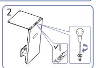
Put the stand base onto the stand neck as the direction shown in the figure. Check that the stand neck is firmly connected. Tightly fasten the connecting screw at the bottom of the stand base.
