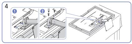
Push the assembled stand into the main body in the direction of the arrow as shown in the figure. Tightly fasten the connecting screw at the bottom of the main body.
