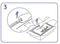
As shown in the figure, remove the product and foam cushion, and then place the product on the table with its front side facing the floor.
