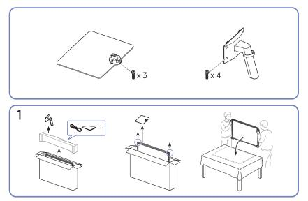
As shown in the figure, remove the product and foam cushion, and then place the product on the table with its front side facing the floor.
