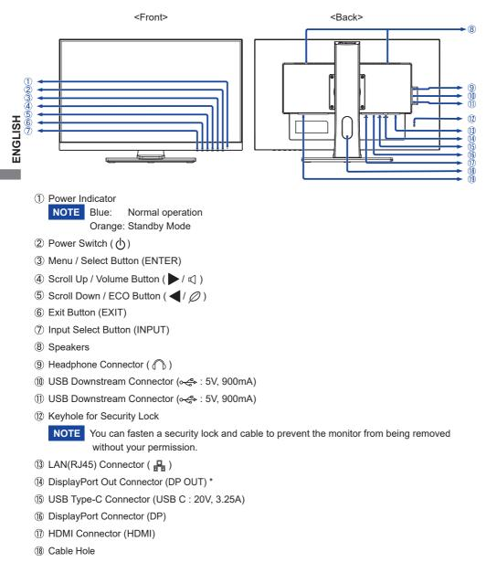
(19) AC Connector (  $\sim$  : Alternating current)
