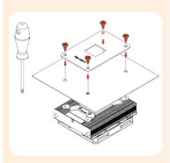
Caution: Gently tighten the screws until they stop, but don't use excessive force (max. torque 0.6 Nm).
