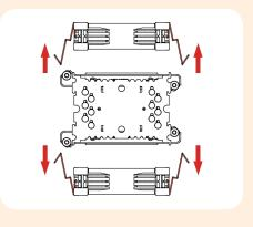
Then put the heatsink onto the CPU so that the four spring-loaded screws align with the threads of the CPU socket. Use the supplied mounting tool to tighten the screws. Perform 3 turns on each screw, then repeat until all are fully tightened.
