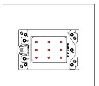
Continue by adding 4 larger drops (5-6mm diameter) of NT-H1 in a square pattern at the center as shown below:
