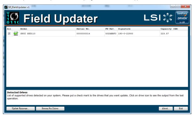
13. Click "Rescan for Drives" to confirm that the SSD firmware has been updated successfully. SF\_FieldUpdater v1 Field Updater DRIVÉN Signature Capacity (GB) SPCC SSD110 505ABBF0 190-0-22900 0000000014 223.57 Detected Drives
