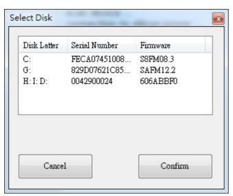
5. After drive selection, the SSD firmware update software will automatically download the corresponding firmware update program.
