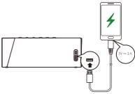
→ The speaker could charge an external device via USB cable.
